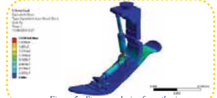
Figure 5 - Stress analysis of prosthesis
